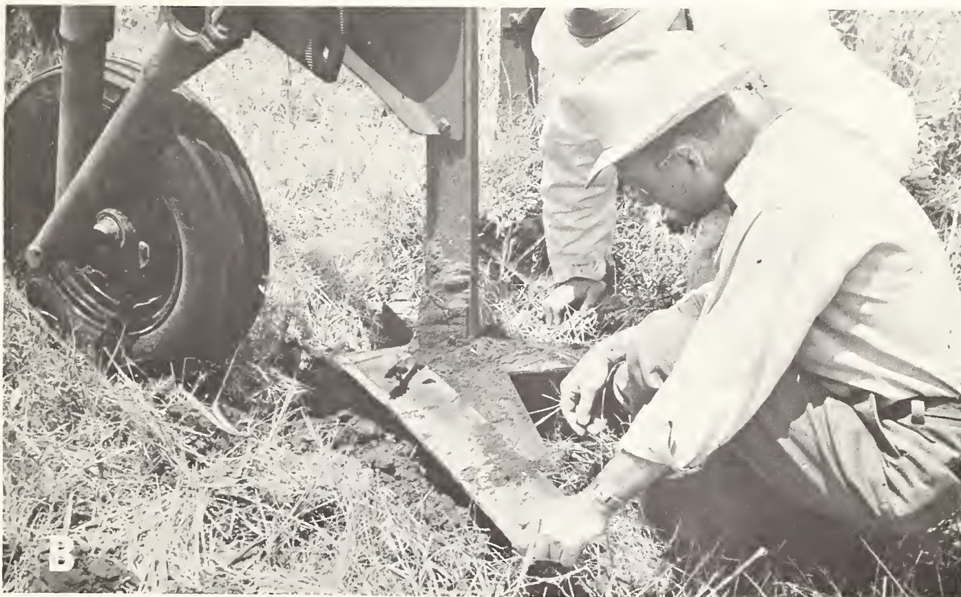
FIGURE 7.—A, Three commercial stubble-mulch plows, connected in a multiple hitch for flexibility, plowing in sorghum stubble in 1950. Total cut was 28½ feet. B, Sweep used on above plows, width 38 inches.
